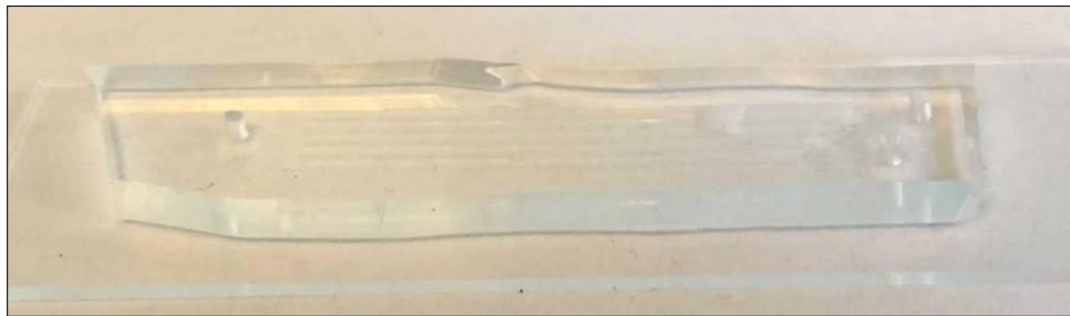
Figure 8: The completed single-height serial dilution module. The glass slide of the device is 25 mm x 75 mm x 1 mm.
