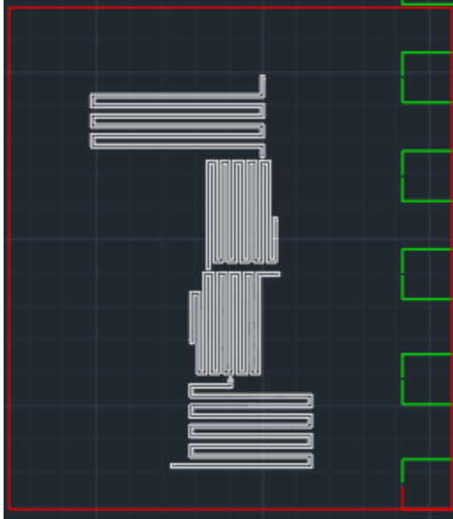
Figure g: Detail of the second layer mask of the double-layer photolithography design (Fig. f).
