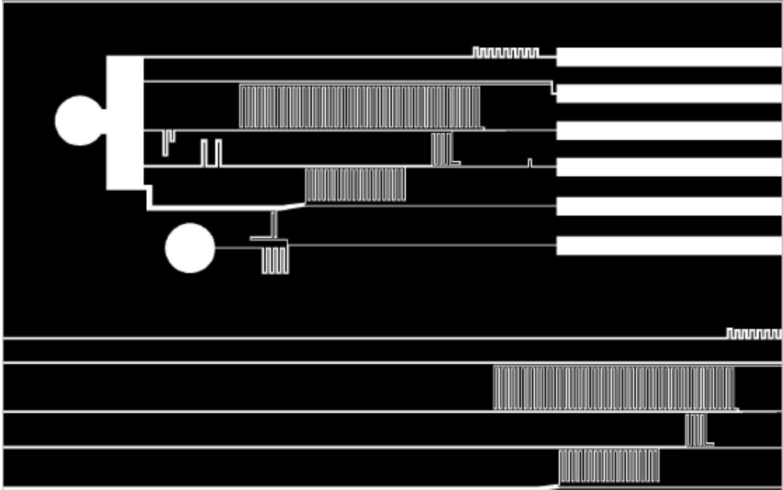
Figure b: Detail 1 closeup of mask design (AutoCAD drawing).
