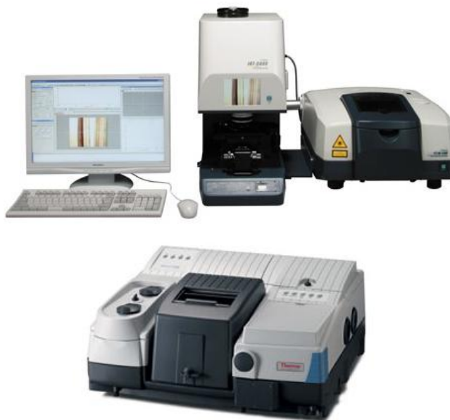
Figure 4.3.2.1: Two types of FTIRs. Left: Jasco Microscope reflection FTIR using a cassegrain lens allowing for reflection measurements averaged at angles from 25 degrees to 45 degrees. [221] Right: Thermoscientific FTIR allowing for normal incident transmission measurements and near normal reflection measurements (10 degrees). [222]
