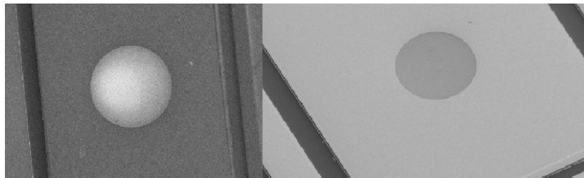
Figure 4.3.1.2: Left: inlens detector used to image a GaSb aperture surrounded by Au. Right: SE2 detector used to image the same aperture.
