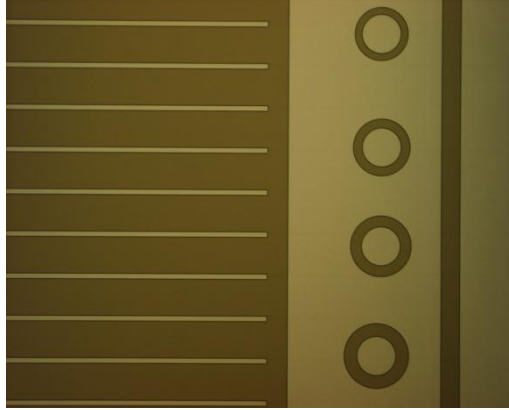
Figure 4.2.2.5: Metallization patterned using photolithography. Light pattern is gold, darker pattern is the GaSb semiconductor substrate after removal of photoresist.
