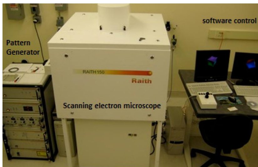
Figure 4.2.3.1: Raith 150 electron beam lithography system. The system includes software controlled pattern generator, field effect scanning electron microscope, and 20 keV electron source. [217]
