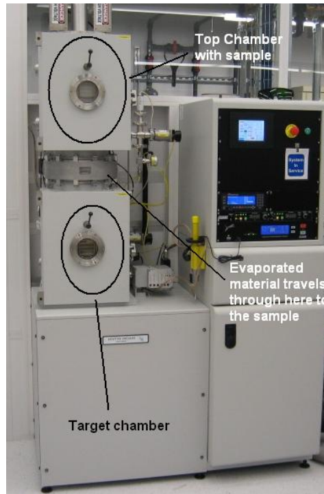
Figure 4.2.4.1: Denton E-beam evaporator. The sample chamber, target chamber, and connector are indicated. [218]
