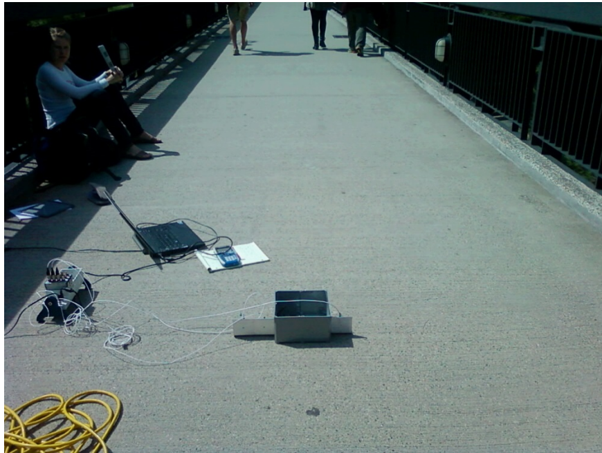
Figure 30: Setup for Test 3 (Sensors at Center of Bridge)
