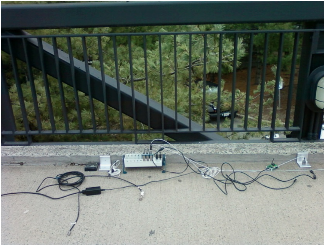
Figure 28: PCB Accelerometers in Test 2 (Right Side of the Bridge)
