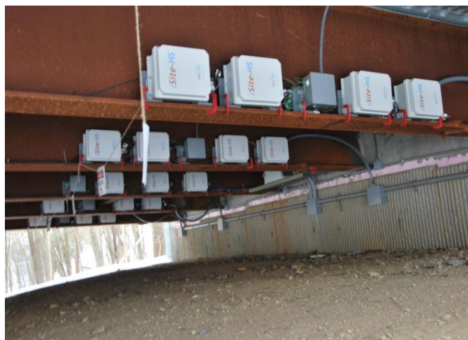
Figure 2.2.2 Data Acquisition System under the PMB
