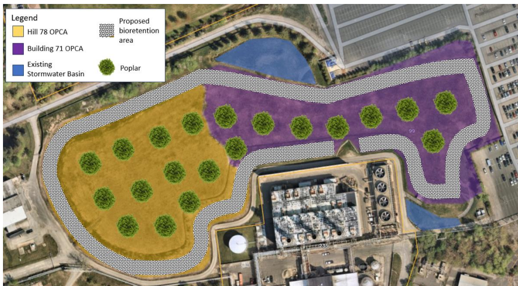
Figure 16: A rendering of a potential bioremediation plan for the Hill 78 and Building 71 OPCAs. Note: tree placement is illustrative and not to scale.
