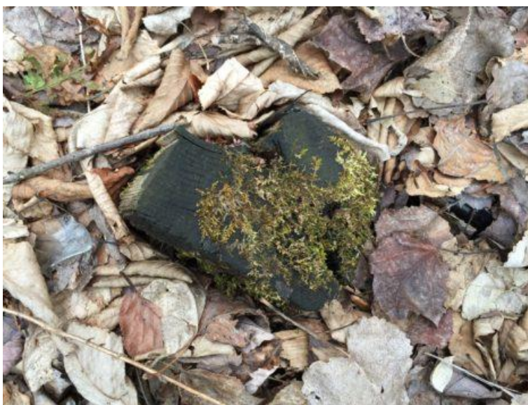
Figure 10: A PCB-saturated creosote brick in Brattle Brook Park. Source: Heather Bellow, Berkshire Edge, 2016.
