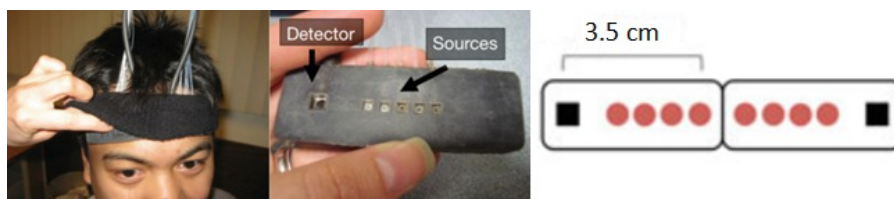
Figure 1. Each fNIRS probe had 4 sources (five are shown but four were used) and one detector which were placed on the forehead to take measurements from the prefrontal cortex. 26
