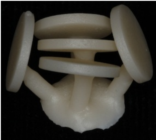
Figure 3: (A) Wax patterns sprued to ring former, (B) Investment filled into the ring.
