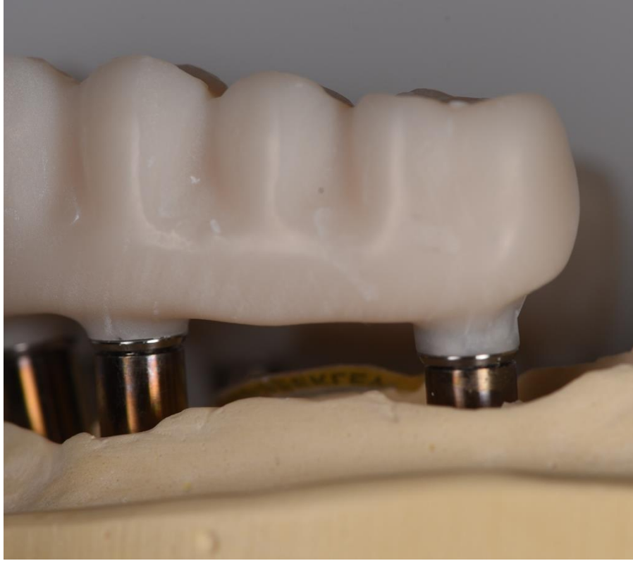
Figure 9. Non-accurate fit is shown with the gap between the printed prosthesis prototype and multiunit abutments (SARS).
