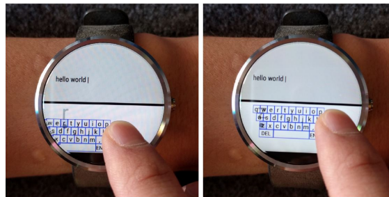
Figure 2. DriftBoard on a Motorola Moto 360 smartwatch with a round display. Left: The fixed cursor is on top of "r". Right: The cursor remains fixed, but acquires "z" due to keyboard movement. A finger-up at this time enters "z". Note that the size of the movable keyboard is not necessarily the same as the device's display. Note also that DriftBoard is applicable to non-rectangular shapes.
