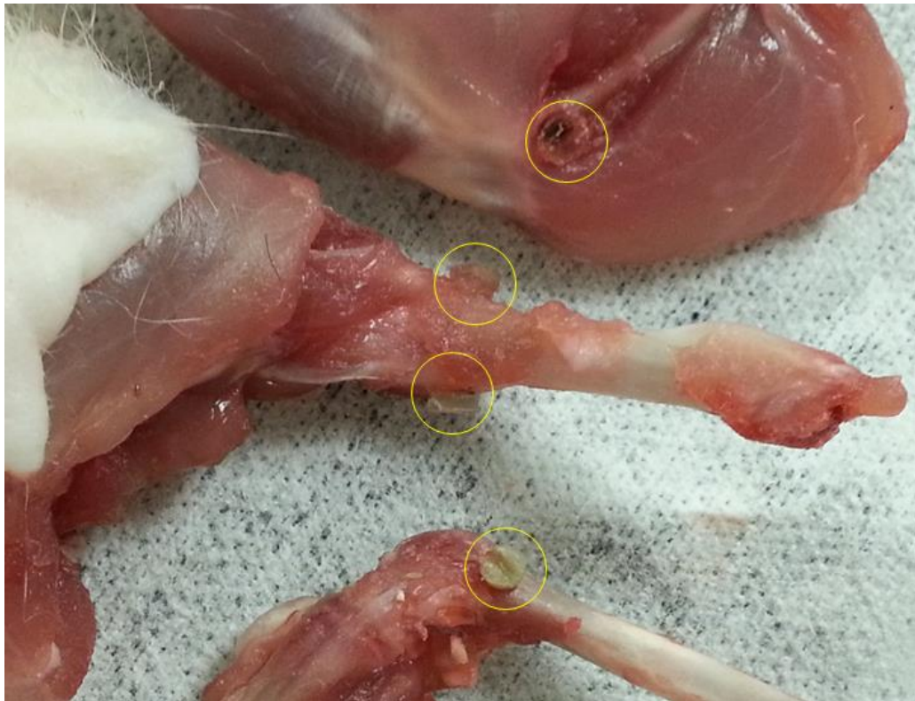
Figure 26 – 1-72 silk screws inserted into cadaver rat femurs. The yellow circles denote the location of the silk screws in the femurs.
