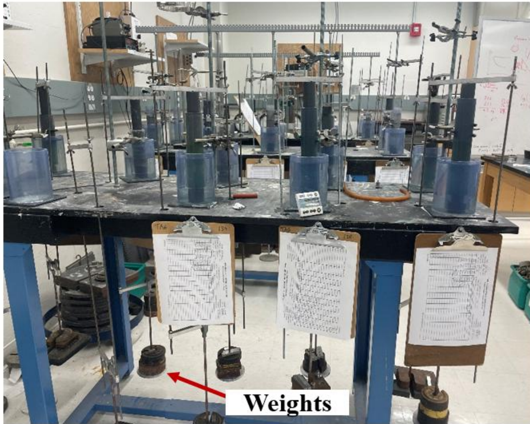
Figure 3.15: A photo from the TAG lab showing a suite of resedimented specimens of glauconite sand and glauconite clay, prepared at different fines contents. Observe the weights that are applied to consolidate the specimens to the desired effective stress.
