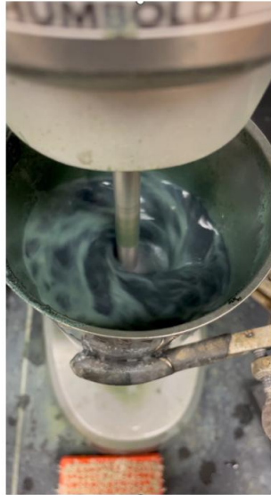
Figure 3.13: Two photos of different glauconite sand crushing methods. The left photo is glauconite sand that is being sheared in the Humbolt malt mixer. The right photo is a wrist-action shaker is being used to crush glauconite sand with ceramic balls in plastic bottles.
