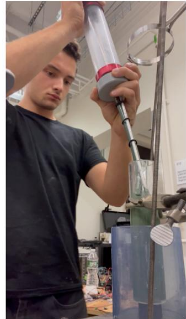
Figure 3.14: The resedimentation process, developed by the TAG Lab is summarized here in three photos. Left: First the glauconite sand and clay are mixed at the desired fines content, salinity, and water content. Middle: After mixing sufficiently, the soil slurry is de-aired using a vacuum. Right: the author used a syringe to deposit the de-aired soil slurry atop a porous stone and filter paper within a lubricated resedimentation tube.
