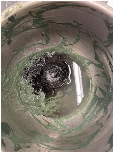
Figure 3.14: The resedimentation process, developed by the TAG Lab is summarized here in three photos. Left: First the glauconite sand and clay are mixed at the desired fines content, salinity, and water content. Middle: After mixing sufficiently, the soil slurry is de-aired using a vacuum. Right: the author used a syringe to deposit the de-aired soil slurry atop a porous stone and filter paper within a lubricated resedimentation tube.
