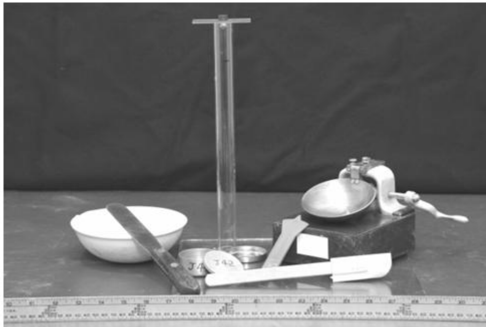
Figure 5.2: A picture of the Casagrande cup, plastic grooving tool, mixing spatula, water content tares, and resilience tester (Source: Germaine & Germaine 2009).
