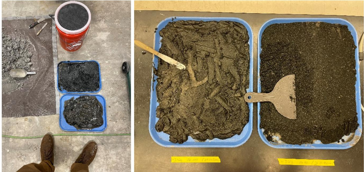
Figure 3.12: Photos from the glauconite sand processing. The left photo shows glauconite marl before and after washing over the stacked sieves. The right is a close-up of the processed glauconite sand before the vacuum filtration method was applied.
