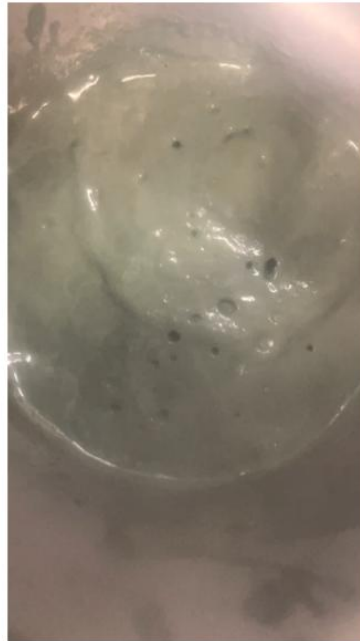
Figure 3.14: The resedimentation process, developed by the TAG Lab is summarized here in three photos. Left: First the glauconite sand and clay are mixed at the desired fines content, salinity, and water content. Middle: After mixing sufficiently, the soil slurry is de-aired using a vacuum. Right: the author used a syringe to deposit the de-aired soil slurry atop a porous stone and filter paper within a lubricated resedimentation tube.
