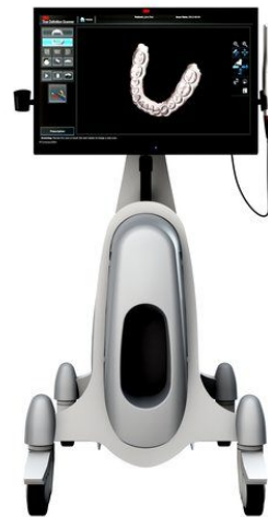
Figure 3. True Definition Intraoral Scanner
