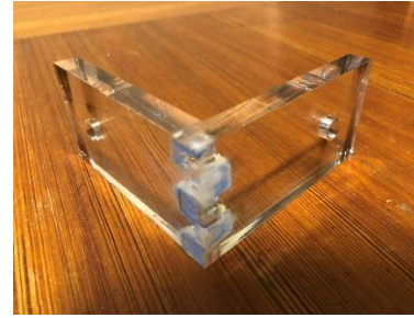
Figure 4-38 Gluing on Finger Joints
