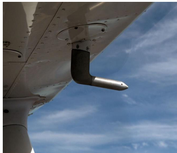
Figure 5-3 Pitot-static Tube on Aircraft taken from Student Pilot News: https://studentpilotnews.com/2019/07/22/quiz-pitot-static-system/
