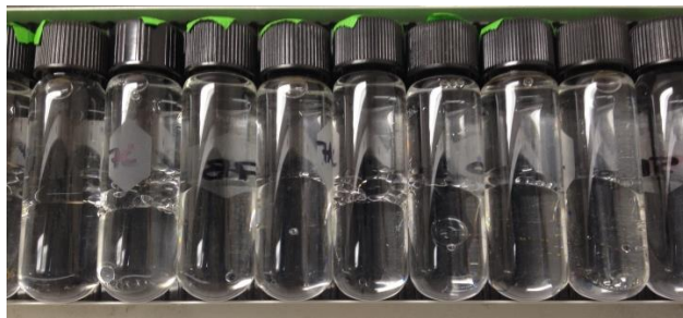
Figure 3.3 Abiotic batch reactors containing a partitioning electron donor and non-aqueous phase liquid, on an oscillating shaker table.
