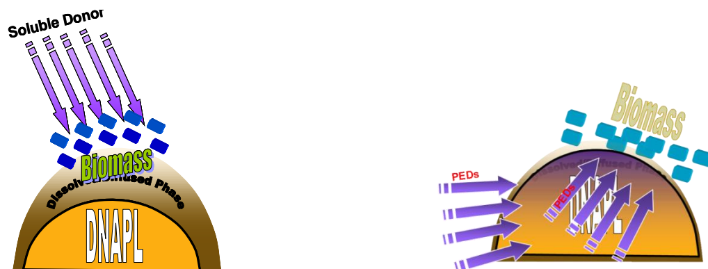
Figure 2.3 The difference between a soluble electron donor and a partitioning electron donor (Cápiro 2012).
