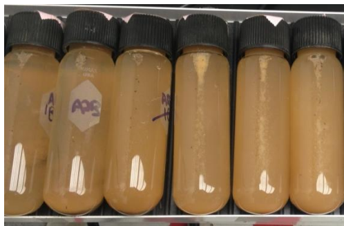
Figure 3.4 Batch reactor containing Applng Soil, mixing on an oscillating shaker table.
