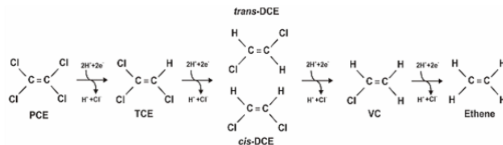
Figure 2.2 Process schematic of biodegradation of PCE to Ethene (ITRC 2008).
