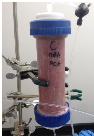
Figure 3.5 Abiotic column containing residual tetrachloroethene dyed with Oil-Red-O.
