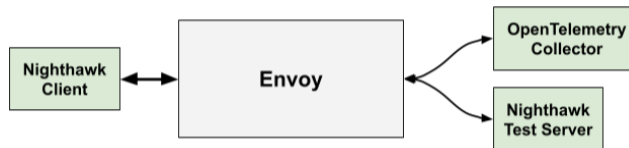
Figure 7. Diagram of the simple test system for evaluation consisting of the Nighthawk Client, Envoy, the Nighthawk Test Server as the single backend, and the OpenTelemetry Collector.
