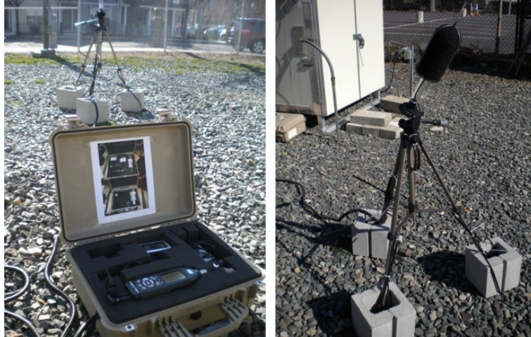
Figure 2. Microphone mounting setup (photo by author)
