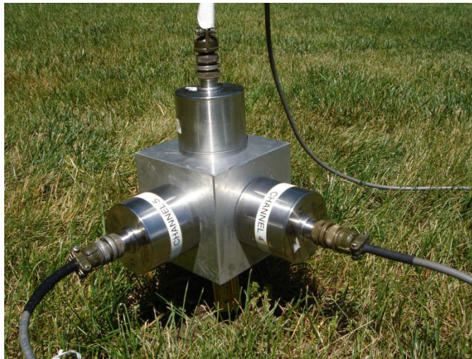
Figure 3.1.3. Tri-axial accelerometer setup in open field
