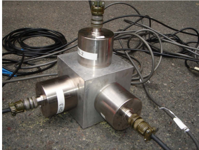
Figure 2.3.1. Tri-axial accelerometer setup
