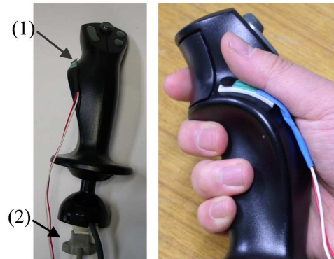
Fig. 3 Spatial mouse with attached FSR (1) and receiver (2).
