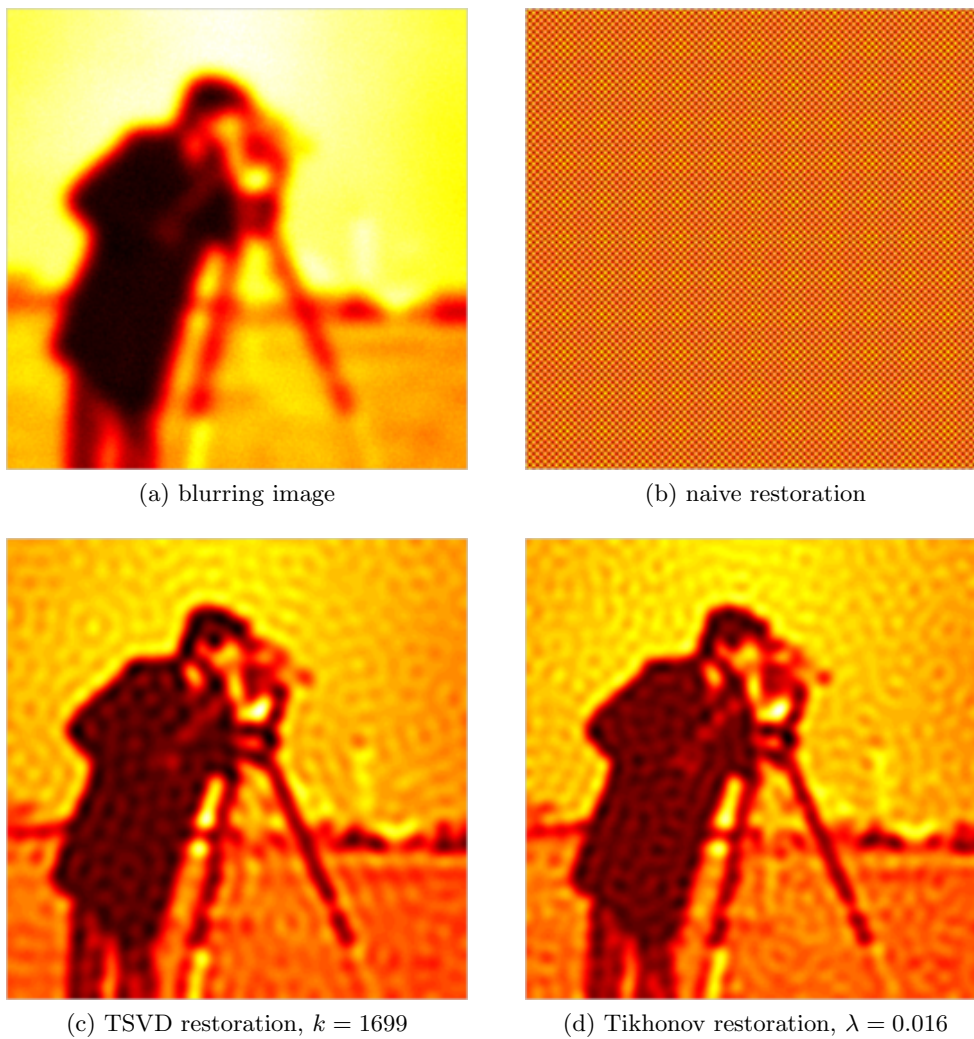
Figure 1.4: Restored images, the regularization parameters in TSVD and Tikhonov methods are chosen with GCV method. (a) blurred and noisy image. (b) naive restored image. (c) restored image by TSVD method. (d) restored image by Tikhonov regularization method.
