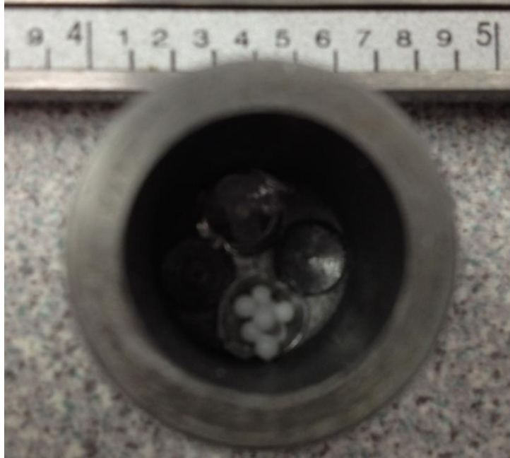
Figure 2: A photo of the custom machined molybdenum crucible, with a metric ruler for scale. Two molybdenum sample cups can be seen in the North and South crucible holes, with the North sample being silica and the South sample alumina.
