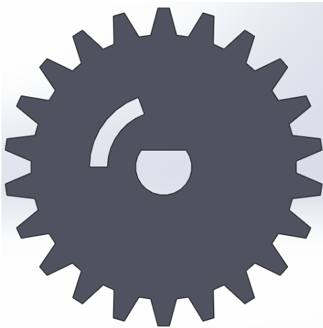
Figure 10: A render of the sighting gear used to isolate one sight tube and allow the four sample cups to be measured using one pyrometer.
