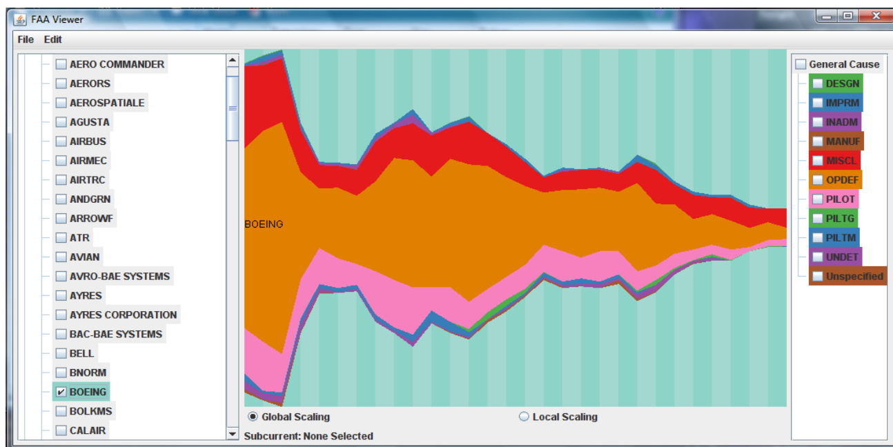
Fig. 1. The 'forward flow' consists of the entire ThemeRiver, showing the number of incidents over time for Boeing (the sole selected category in the 1st dimension.) The 'backward flow' consists of the colored currents within the main river, which show the proportions and trends of categories in the 2nd dimension in the overall river of the selected category in the 1st dimension. Shading lines in the background indicate units of time, in this case years.
