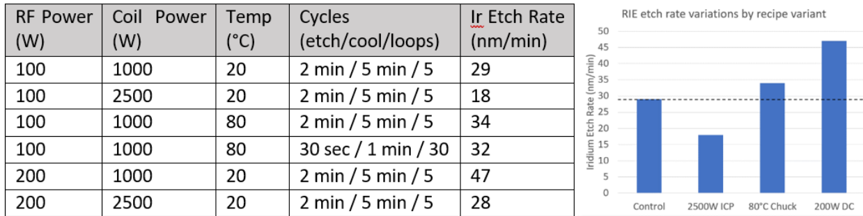
Figure 15. Bar graph of iridium etch rate by RIE recipe variant beside the associated recipe details.
