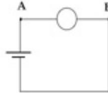
Response #3 is the correct response. Because charge is conserved, the flow of charge (current) through any point in the circuit should be the same.
