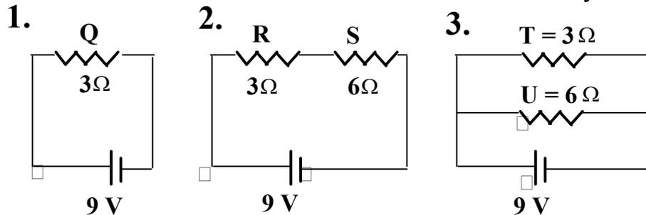
Although circuit number one has the fewest resistors, circuit number three has the smallest equivalent resistance and, thus, the largest current from the battery. Students' comments while discussing this question were coded as follows:
