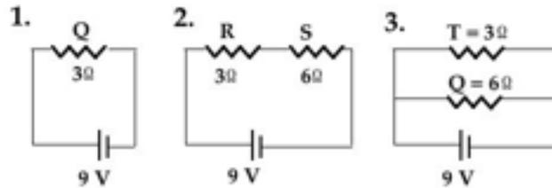
Although circuit 3 has more resistors than circuit 1, their parallel arrangement results in a smaller equivalent resistance and a larger current flow as compared to the other two circuits. The correct response is 3. Student responses are shown in Table 6 below:
