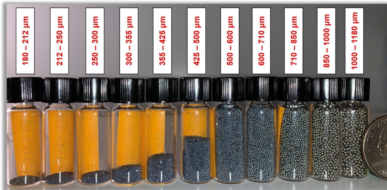
Figure 3-1: Fe-Al samples with distinct particle size ranges between 180 \mu\text{m} and 1180 \mu\text{m} .
