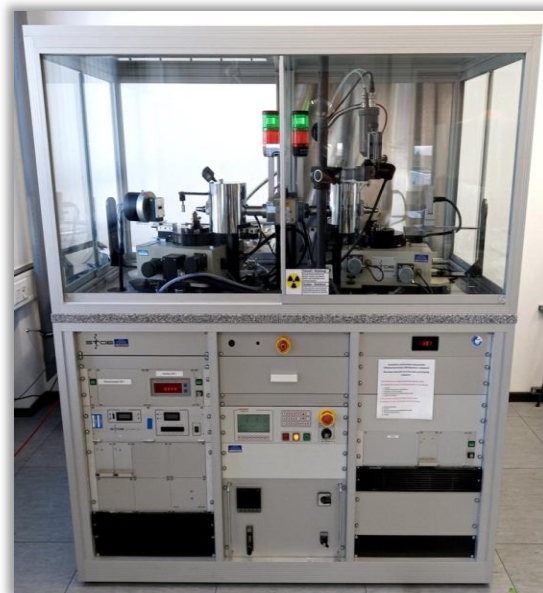
Figure 3-12: Stoe STADI P transmission powder diffractometer located at IFW Dresden. Image reproduced from source [47].
