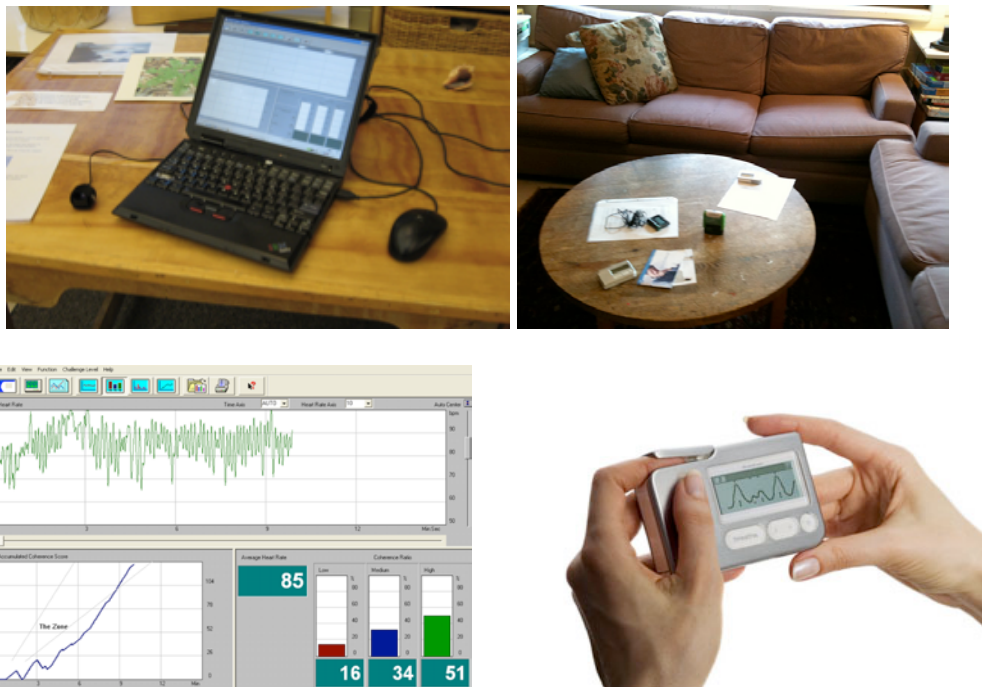
Figure 5. Biofeedback Station. The station offers two versions of heart-rate variability biofeedback activities: FreezeFramer biofeedback software on a laptop computer (left) and StressEraser handheld devices (right).
