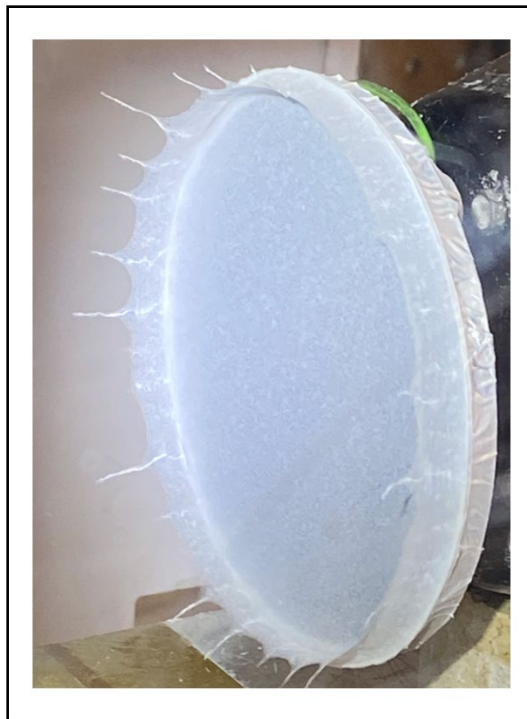
Figure 3.6: Accumulation of fibers along the edge of the collector plate. This is caused when the diameter of the cone shaped whipped fiber jet is greater than the diameter of the collector plate.
