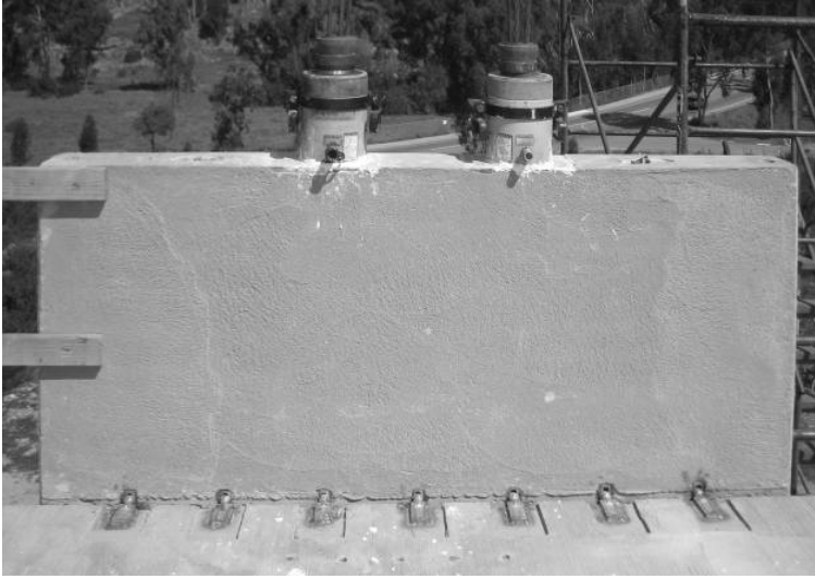
Figure 9 – Floor to wall vertical slotted connections.
