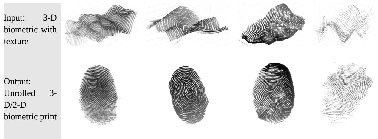
Figure 7.14: Shows the depth fused biometric image and the unrolled 3-D/2-D fingerprints.
