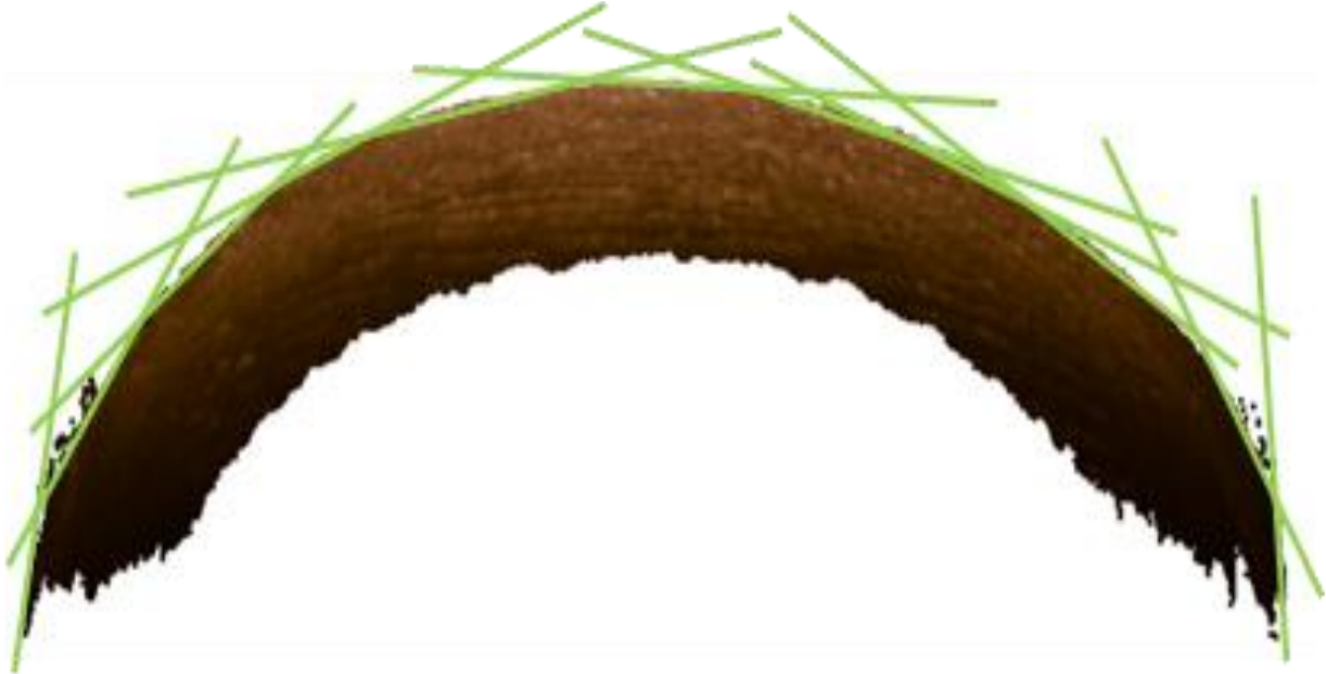
Figure 7.17: Shows the pressure simulation lines. Each line visualized the point of contact while pressure was applied. Pressure will be simulated along the normal of each line. Increasing the number of slices will produce a natural rolling effect but at the cost of a higher computational cost.
