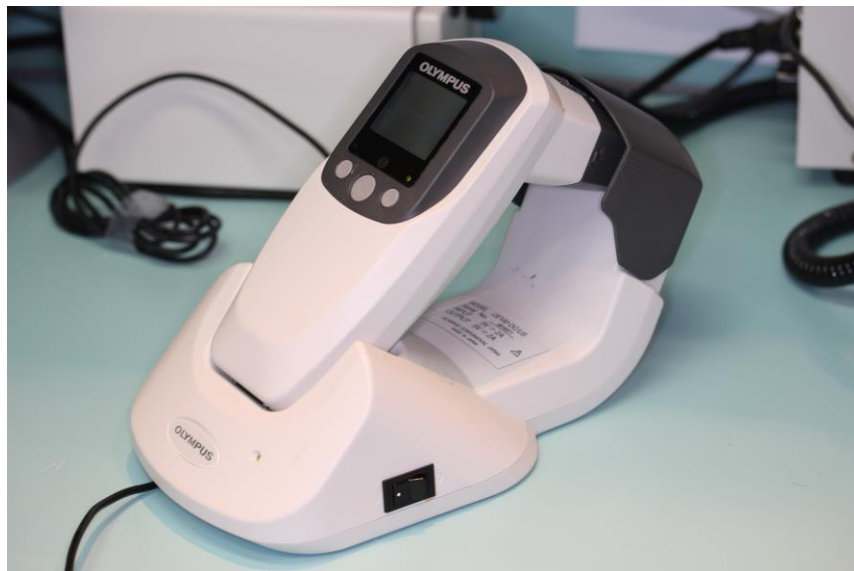
Figure 20: Color assessment using a spectrophotometer, Crystaleye® (Olympus, Shinjuku, Tokyo, Japan). Used to measure dentin hardness (VHN) in three different timings: Phase 1: before demineralization, Phase 2: after demineralization, Phase 3: one week after 2 nd SDF application.
