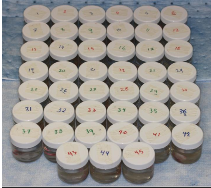
Figure 11: Samples were placed into respective 60 ml jars before applying 40 ml of demineralization solution.
