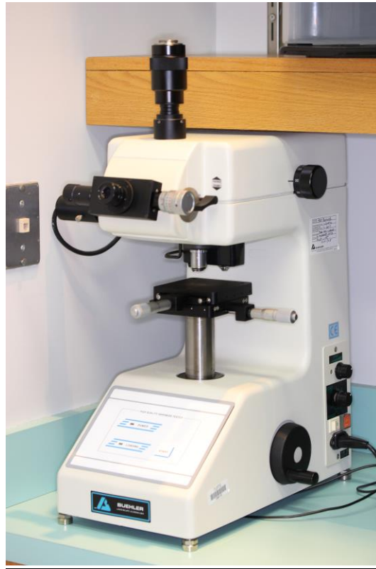
Figure 14: Hardness assessment using (Buehler, Lake Bluff, IL, USA, Wilson VH1202). Used to measure dentin hardness (VHN) in three different timings: Phase 1: before demineralization, Phase 2: after demineralization, Phase 3: one week after 2 nd SDF application.
