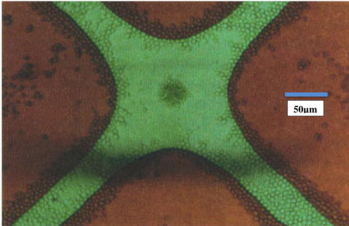
Figure 3.2 Polynomial electrodes for trapping yeast cells. Viable cells are trapped at the electrode surfaces by positive dielectrophoresis while non-viable are trapped in the center by negative dielectrophoresis. The trap was operated at 10 MHz, 5 Vrms. [84]
