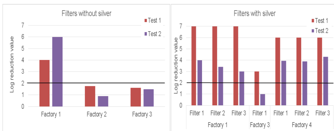
Figure 21: Log reduction values of filters without and with silver application
