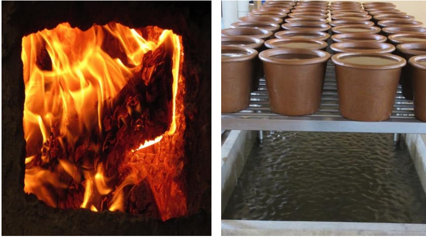
Figure 5: Firing and flow rate testing
