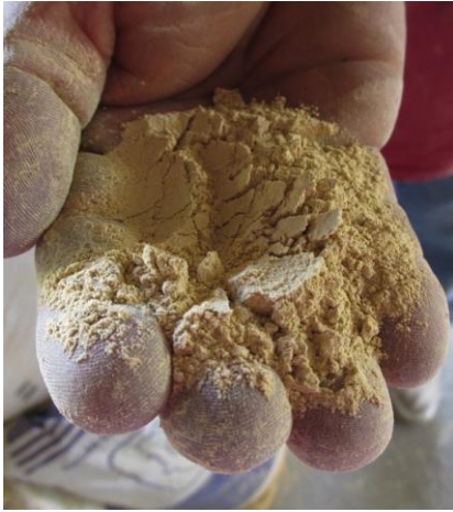
Figure 2: Clay and burn-out material processing
