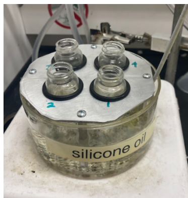
Figure A6.4. Configuration of typical Ag and AgNi colloidal synthesis— the frame ensured that the vials had enough support to be continuously stirred and heated throughout the synthesis period. Design of the frame adapted from Ref 18 .
