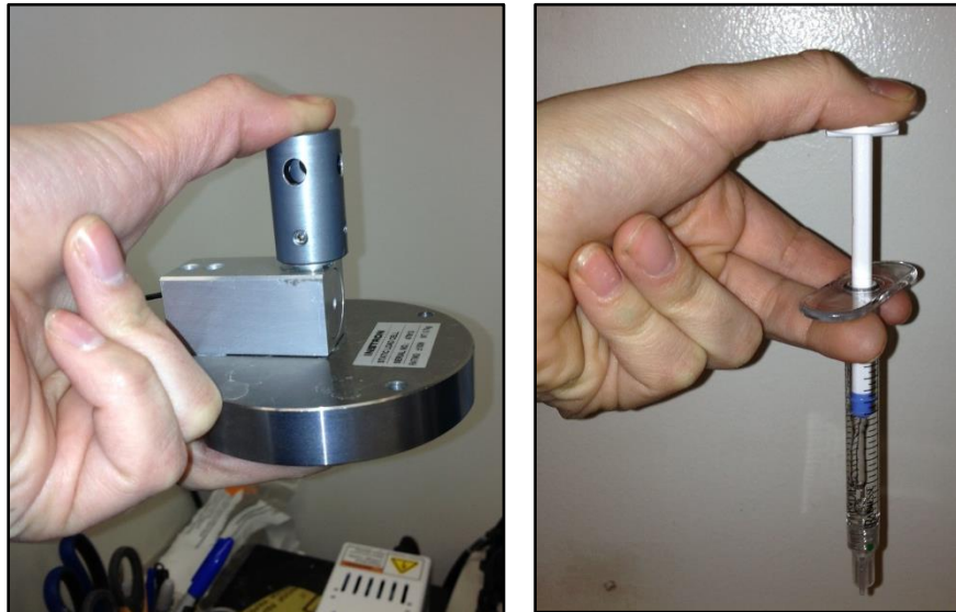
Figure 20: Mechanical compression testing for maximum applied force.
