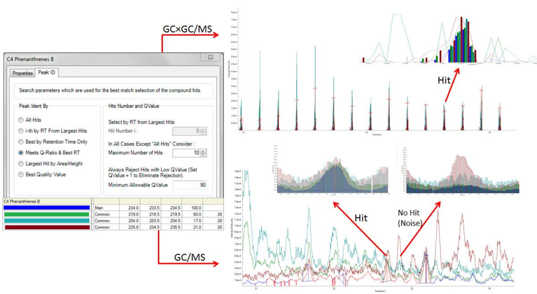
Figure 5-3. Illustrative example of spectral deconvolution of GC/MS and GCxGC/MS data of the coal tar soil shown in Figures 5-1 and 5-2
