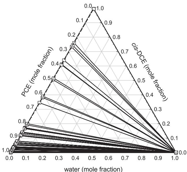
**Figure 1.** Phase diagram for the water/*cis*-DCE/PCE ternary at  $22 \pm 0.1^\circ\text{C}$  with measured tie-lines (solid lines connecting squares), and UNIFAC prediction of binodal curves (dashed line).
