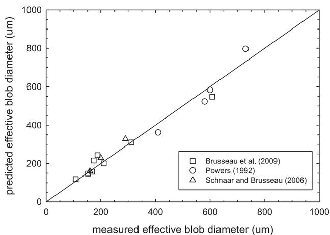
**Figure 3.** Measured versus predicted blob diameters using the correlation shown in equation (12).
