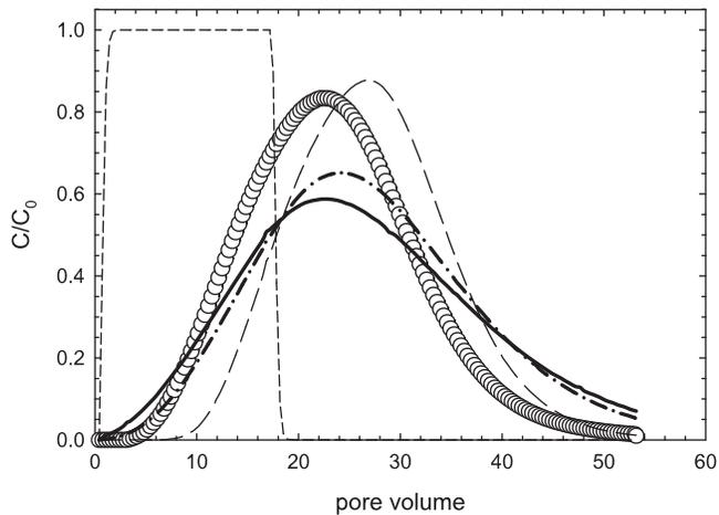
**Figure 4.** Normalized effluent concentrations of *cis*-DCE and model predictions for Column A: data (circles), non-reactive pulse (short dashes), local equilibrium assumption (long dashes, 0.161), rate limited with Powers *et al.* [1992] correlation (solid line, 0.129) and rate limited with Imhoff *et al.* [1994] correlation (dashes and dots, 0.120). Numerical values represent the root mean square differences between the data and each simulation of *cis*-DCE partitioning.
