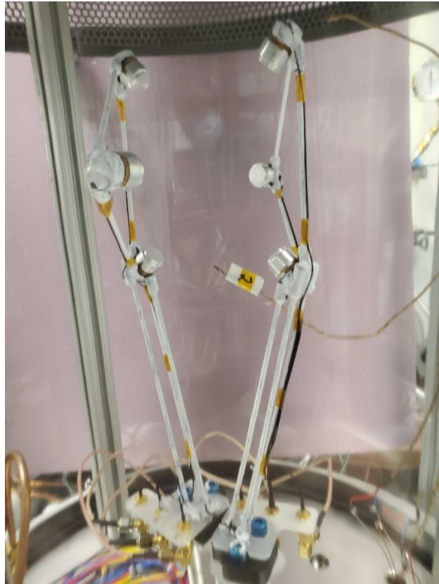
Figure 32, Bell jar testing of an octahedral without every edge.
