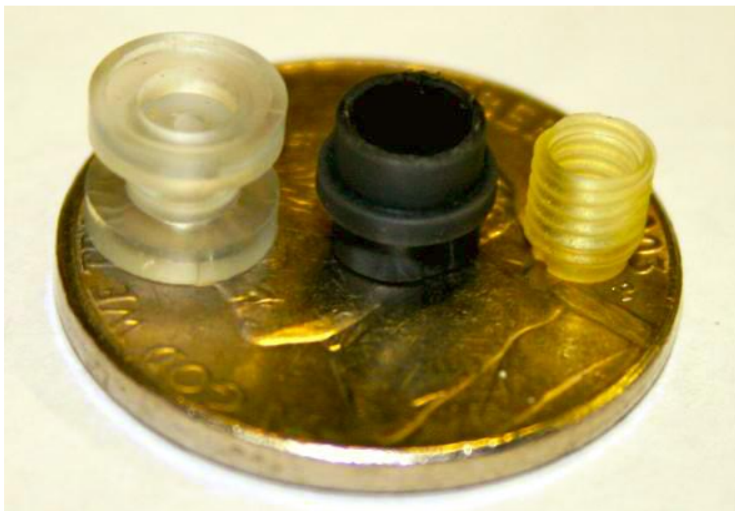
Figure 5.3. Size comparison of the housings proposed all placed on a nickel. On the far left is the WCL/RCAL type housing, in the middle is an intermediate design for CHEMSENS, with the housing on the far right being the final CHEMSENS threaded housing with an O.D. ~4 mm.
