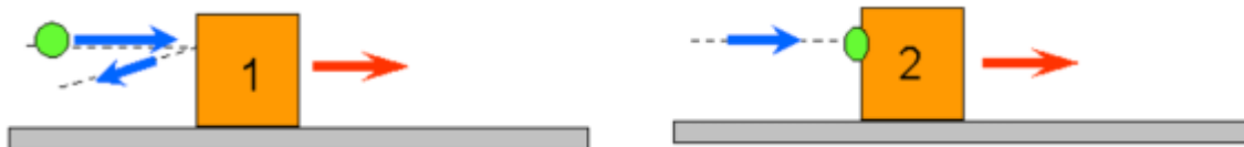
Figure 4.2: Two balls of equal mass are thrown horizontally with the same initial velocity. They hit identical stationary boxes resting on a frictionless horizontal surface. The ball hitting box 1 bounces back, while the ball hitting box 2 gets stuck. Which box ends up moving faster? (Unit 11)
