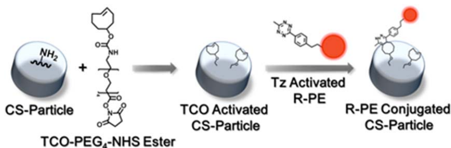
Figure 4.2. Schematic diagram for TCO activation of the CS-particle via an amine-reactive chemistry and R-PE conjugation with the TCO-activated CS-particle via Tz–TCO cycloaddition reaction.
