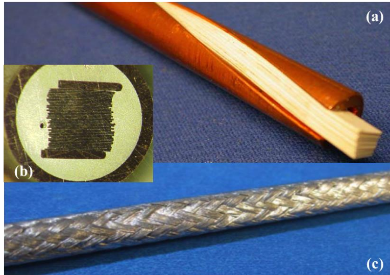
Figure 2.3 – Images of different twisted stacked-tape cable variations [18]. TSTC in a solid copper core (a), a solder filled copper tube (b) and a braided copper sleeve (c).
