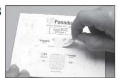
Lift one end of horizontal graph paper and peel it slowly from backing sheet.
