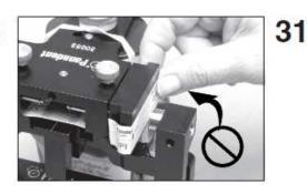
After marking graph paper, lock graph support in contact with side of maxillary frame with thumbscrew.
