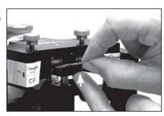
Place marking ribbon (dye toward graph paper) with index finger and thumb of one hand. Mark horizontal graph by lifting up on distal end of graph support with index finger of other hand (vertical arrow).
