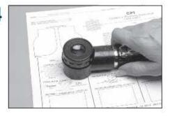
OPTIONAL: Use optical resolver (10x) and illuminator to read graph markings accurately with 0.1mm reticle scale in resolver.
