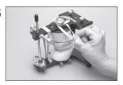
In preparation for removing casts from CPI, release and remove the two lateral elastic support bands from their associated retainer pins below mandibular cast.
