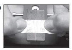
Stretch horizontal graph paper laterally with thumbs and index fingers. Align heavy center line of paper with center line of graph support. (Anterior-posterior position is not critical.)
