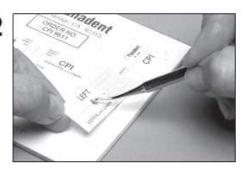
With small-ended dental instrument (e.g. Tanner carver), lift one end of vertical graph paper. Grasp free end of graph paper with thumb and index finger. Press tip of dental instrument against rectangular cut-outs on graph paper while slowly peeling adhesive coated paper from backing sheet. (Two small rectangular cut-outs should remain attached to backing sheet after graph paper has been removed.)
