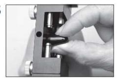
Press protector cap completely over horizontal graph marking pin.
