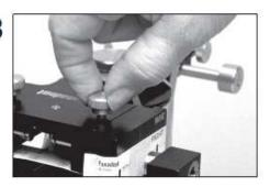
Loosen locking thumbscrew for vertical graph support in preparation for marking vertical graph.
