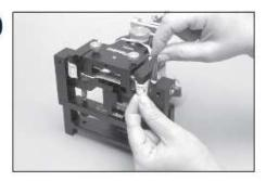
Place single sided marking ribbon over graph paper (dye toward paper) with fingers of one hand. Grasp <u>distal end</u> of graph support with thumb and index finger of other hand for marking graph paper.
