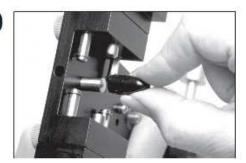
Pull soft plastic protector cap from marking pin for horizontal graph.
