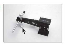
Place maxillary frame on right side graph support for placing left vertical graph paper. Note anterior end of frame resting on "foot" of transverse support post (arrow).
