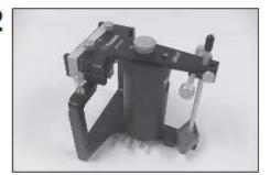
Maxillary and mandibular CPI frames joined together with inter-frame support column
