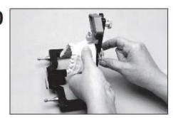
Attach interchangeable articulator mounted mandibular cast to lower frame of CPI with mounting plate thumbscrew (or magnetic mounting plate).
