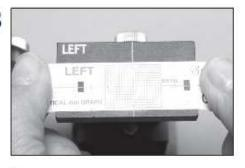
Hold both ends of graph paper with thumbs and index fingers. Brace index fingers against anterior and posterior ends of graph support and stretch paper tightly. Align both vertical and horizontal cross lines of paper with cross lines on graph support. After final alignment is complete, apply light finger pressure to adhere paper firmly to graph support.
