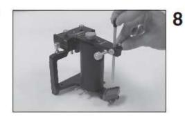
Loosen mounting plate thumbscrew and remove maxillary frame from inter-frame support column. Do not force or bind precision locating dowels when removing frame from support column.
