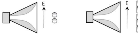
Figure 32: Orientation of resonators in reference to antenna. Note direction of E field. The resonator pair and five-element array are oriented in different directions.
