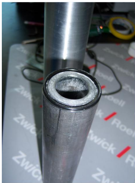
Figure 2.4: The static o-ring was designed to prevent the permeation of the force transmission medium into the annulus between the test section and test housing.
