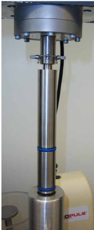
Figure 2.5: The dynamic o-ring installed on the load piston set was designed to prevent the force transmission fluid from displacing upward during testing.
