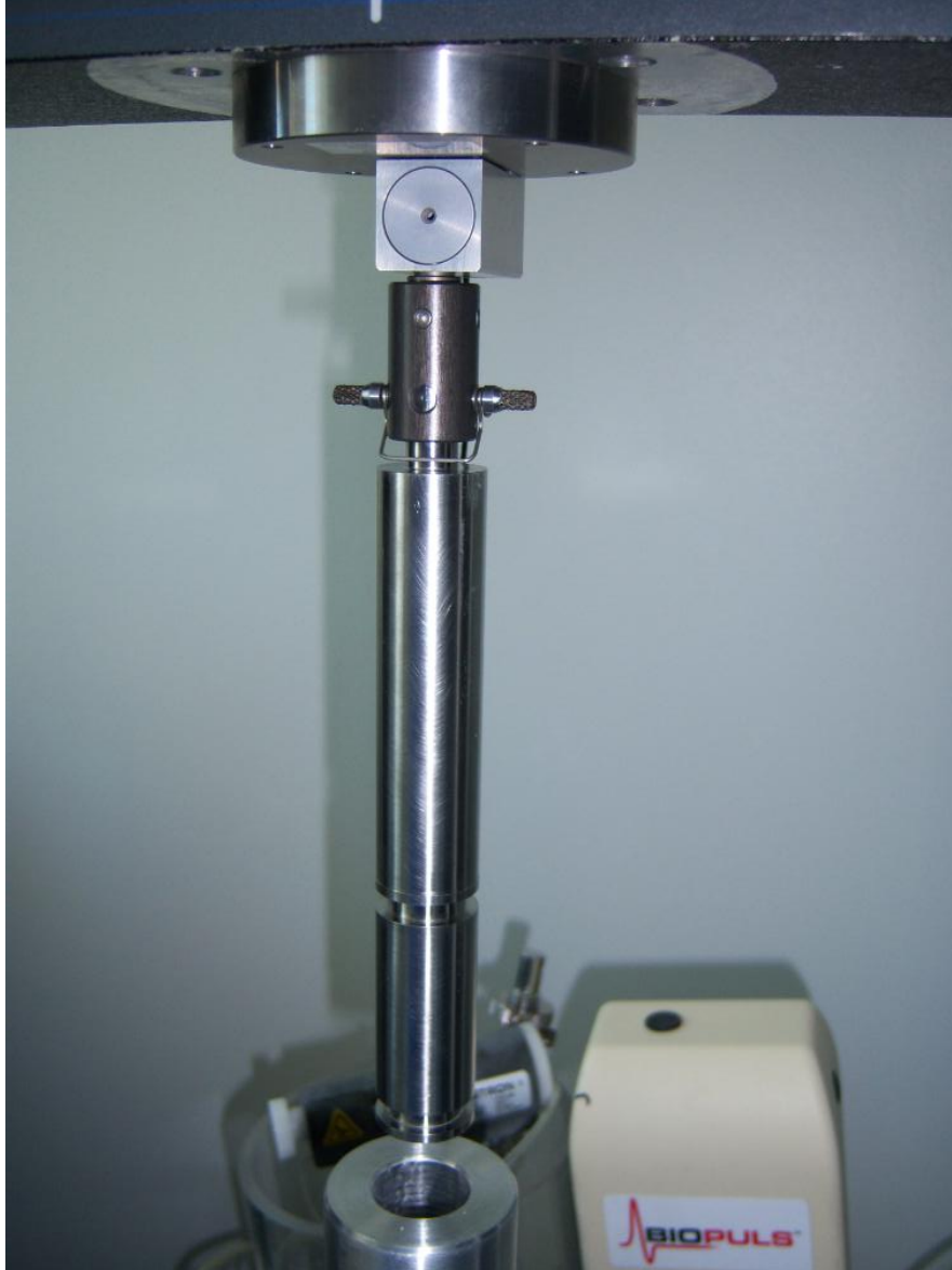
Figure 2.2: The load piston can be attached to the load cell through the use of 6mm Clovis pin connection.
