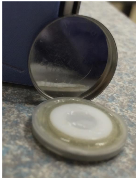
Figure 2.5.1 Cell tester assembly for measuring the room temperature ionic conductivity of the sample.
