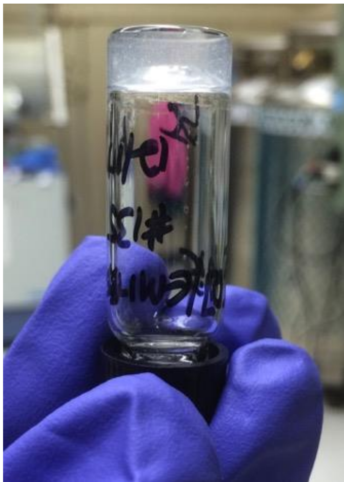
Figure 2.2.2 Typical gel sample showing no flow upon vial inversion
