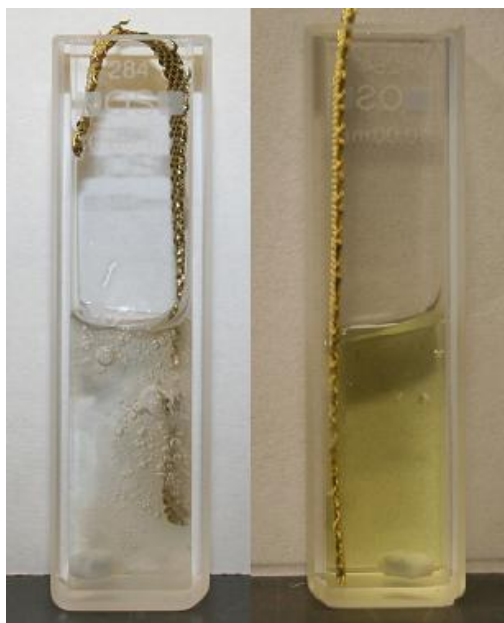
Figure 18. Completed activity assays of 1:50 mass ratio of OPH to chitosan film. Left: Chitosan film expands and OPH activity is not observed. Right: Chitosan film did not expand as much compared to the left figure and activity was observed.
