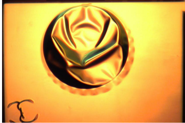
Figure 5-2 Image of Cr/Au blister caused by compressive stress within the multi layered film.
