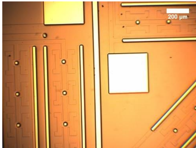
Figure 6-2 50 nm/ 4 μm of sputtered Ti/Cu in the NSC3000 sputter tool.
