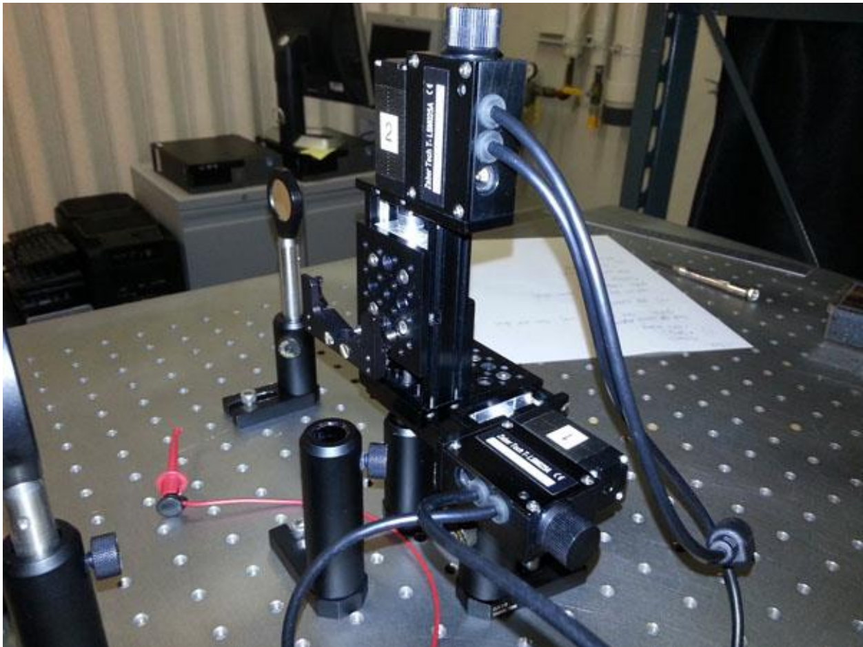
Figure 4: Two linear stages are combined to form the XY stage. The knobs allow for manual adjustment of the stages.
