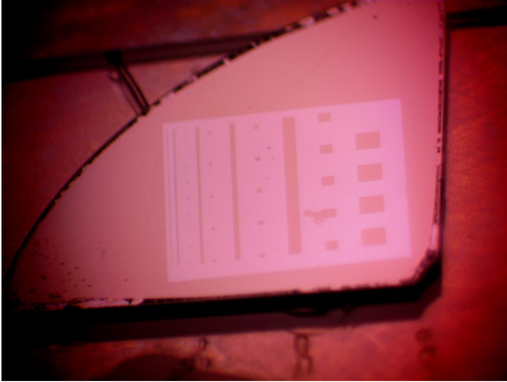
Figure 7: This image was taken at an angle with a diffuse incandescent light source reflecting off the sample into the camera. This direct reflection allows us to differentiate the darker chrome areas from the lighter GaAs regions.
