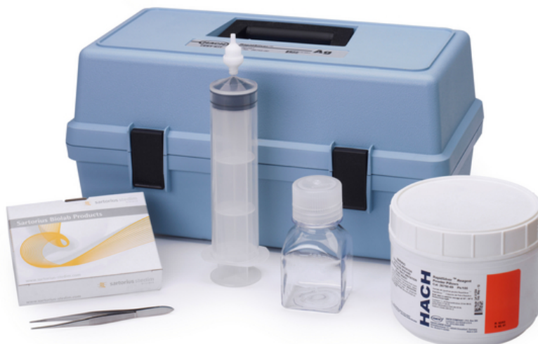
Figure 5. Hach RapidSilver Visual Test kit with (L-R) filter box, forceps, 140 cc syringe and filter holder, 100 mL mixing bottle, and indicator reagent.
