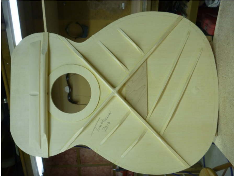
Figure 1.4 Bracing on the back of the top plate (source: http://mullinguitars.com )
