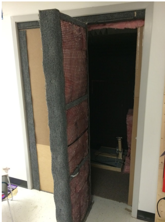
Figure 3.2.2 Quiet chamber built for the frequency response measurement
