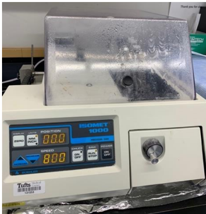
Figure 9: Slicing mounted samples vertically using slow-speed saw with a water-cooled diamond blade IsoMet 1000 (Buehler, Lake Bluff, IL., USA)
