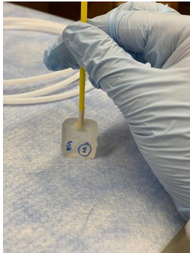
Figure 11: Microbrush used as a plunger for the restorative material, all samples after receiving the restorative material button.
