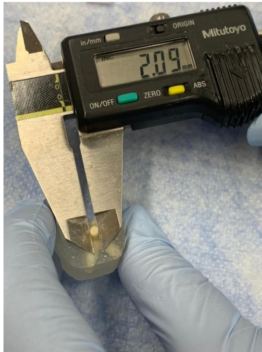
Figure 12: Digital caliper used to confirm diameter of the restoration.
